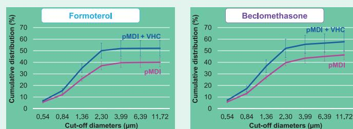
Figure 2: Cumulative distributions with or without VHC of Formoterol and Beclomethasone aerosols from Innovair.
