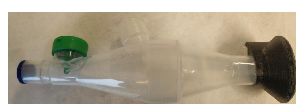
Figure 3 : NeonatHal® prototype inhalation chamber (Laboratoire OptimHal-ProtecSom) with its prototype facemask (created with CAO software (SolidWorks, Dassault System) and 3D printed).
